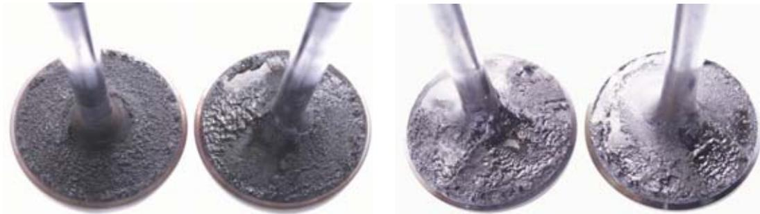
*Fig. 3. Intake valve deposits – Mercedes-Benz M102E, OHC, 2 – VPC, electromechanical Port Fuel Injection [INiG]*
