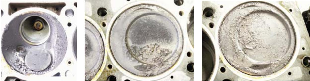
*Fig. 9. Examples of deposit flaking in combustion chamber and on the piston top [INiG]*
